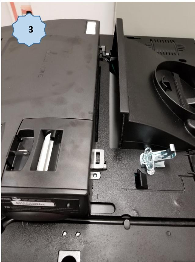
Slide unit forward and remove jammed ballot.
