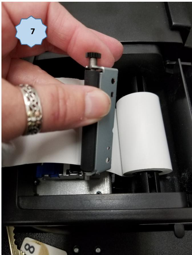
Remove security bar. NOTE: Pay close attention to how it was positioned. Insert new roll of paper.
