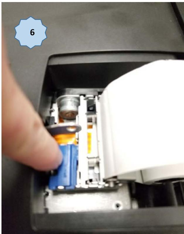
Push blue tab to release the security bar that holds paper in place.
