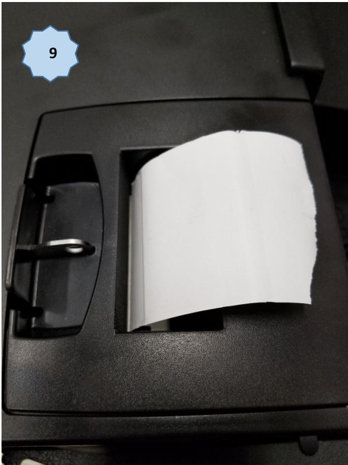
Feed end of paper into slot then close door.
