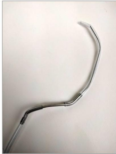
5. Detach the mouth tube by working its lower end gently back and forth until it slips off the metal tube.
