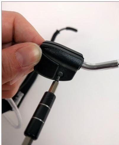
3. Note the position of the tubing inside the bracket. Then remove the mouth tube from the bracket.
