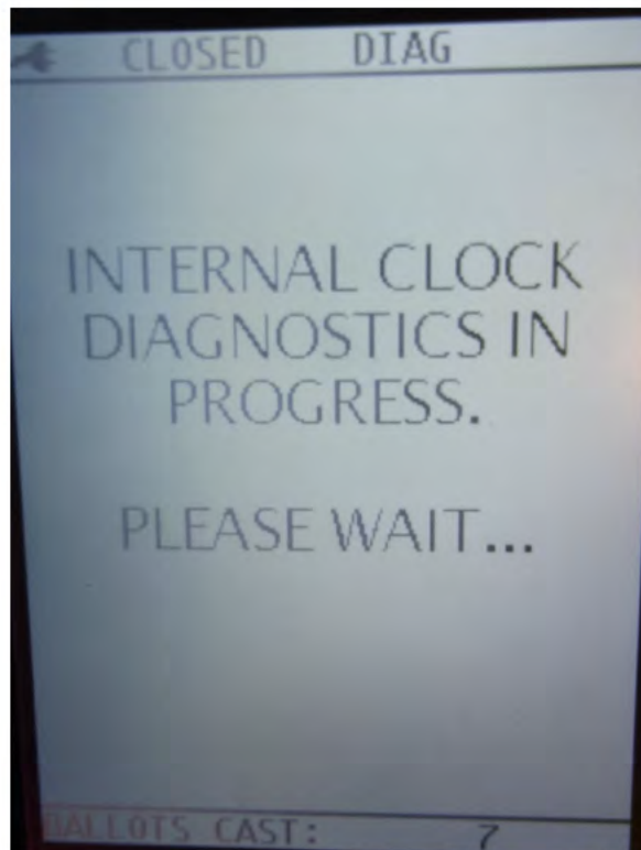
Figure 7 - ICP LCD Clock Diagnostic
